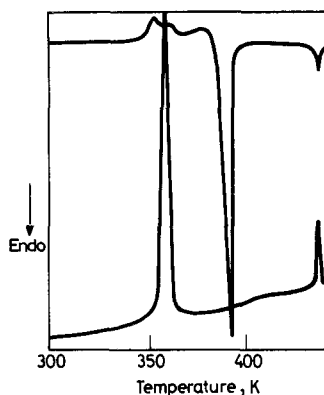
Fig. 7 DSC curves of DB_2-DB_3 equimolar mixture. cooling and b = subsequent heating run
